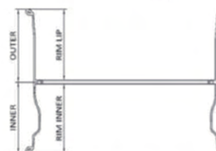
REVERSE Mold Front and Rear ROLL LIP (F)
