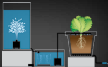
Run to waste system
