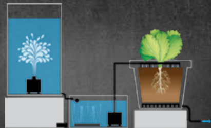
Run to waste system
