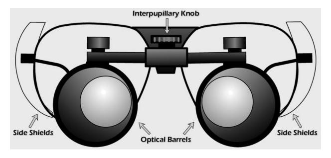
The components of the loupes as shown. The *Interpupillary Knob* adjusts the lateral distance from one barrel to the other. This should be the ONLY adjustment you will need to make. This knob does not need to be adjusted each time you use your loupes. Once set properly, it will not need readjustment.
