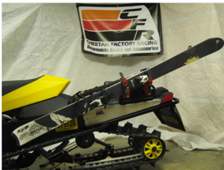
A pair of skis and poles with the tails on the running boards. Note the DD rack must be mounted 12 inches back from seat as shown. This will allow the rear binding clearance from snowmobile.
