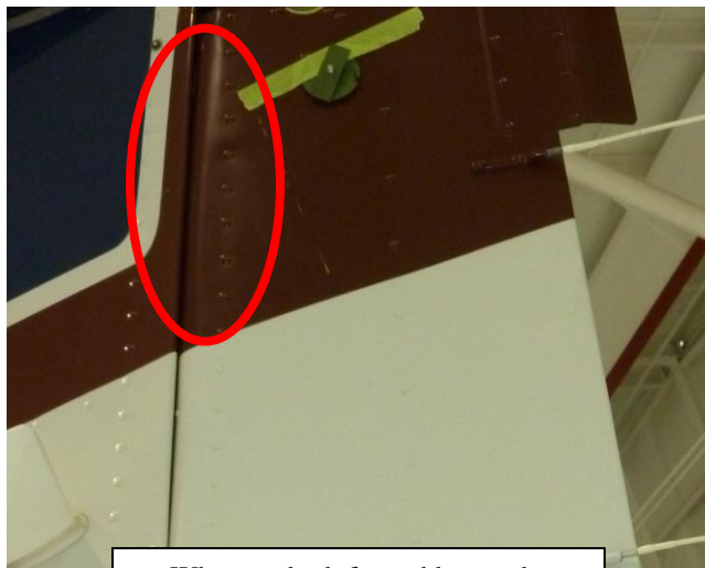
Where to look for rudder cracks
