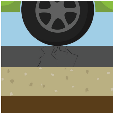
Cracks are formed in road through repeated traffic loading & utility cuts.
