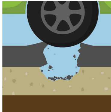
Weight of traffic collapses the road surface into the gap forming the pothole.
