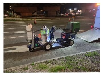
There are many benefits to be found when using cold applied MMA for line marking, compared to using thermoplastics.
