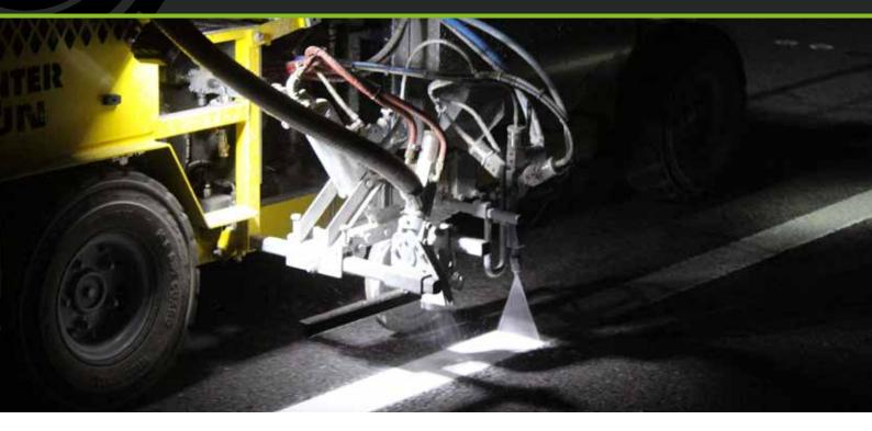
Swarcolux 125-2000 Reactive Glass Beads are hardener coated glass microspheres which are used as the hardening element in 2 component cold-spray plastic marking systems. These glass beads can be used with applications of up to 1.2mm thickness. These beads provide a dual purpose, giving reflectivity to a line as well as being the curing component.
