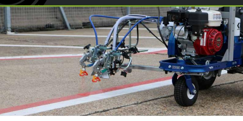
The Graco LineLazer V 200DC machine is ideal for smaller dual colour jobs, simplifying the 2-colour application process. This machine can improve efficiency and profitability by eliminating the need for seperate colour machines or changing colour in a machine, while spending less time refilling materials. Alternatively, it can be used for wide line applications to over 900mm wide. Compatible with LineDriver or LineDriver ES.
