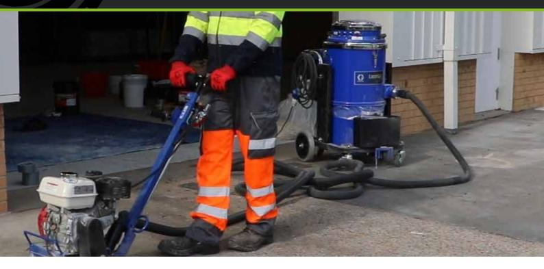
The LazerVac 330 is a highly effective vacuum system for use with the GrindLazer range to reduce airborne silica dust. This system helps meet OSHA's safety requirements for airbourne silica dust and prevents the operator from inhaling harmful dust.
