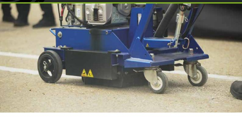
The Graco GrindLazer RC813 G is a rotary scarifier, ideal for line removal leaving no grooves in the substrate. The rotary action of this scarifier hovers over the surface, removing the marking whilst minimising damage to the substrate - making this the "no-groove line eraser." The RC813 G can be linked up to the LazerVac system to reduce airborne silica dust.
