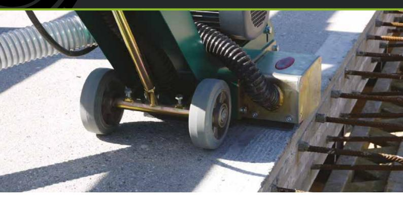
Quality and reliability for high performance and cost effective operation from CONTEC®! The proven Planer CT 200 with either an electric motor, or petrol engine which is ideal for construction sites without power supply. Surface texturing, scabbling, planing, grooving, cleaning, descaling and removal of road markings all possible with the CT 200 or CT 200 P.
