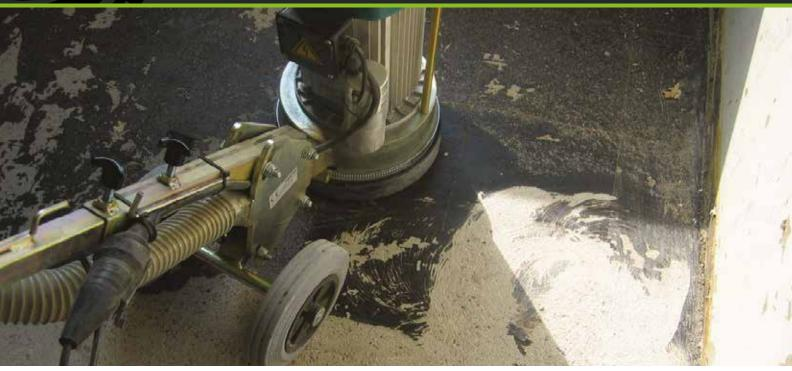
A small grinder with incredible performance! Powered by only 110V or 230V single phase motor, the Alpha grinder reaches the class of 3 phase machines with the weight of only 44kg. Excellent for the removal of existing line markings or floor tape.
