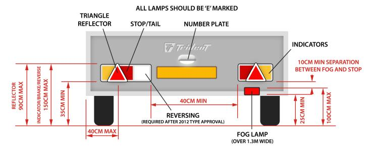
Making sure your trailer has the correct lighting is a legal requirement under The Road Vehicles Lighting Regulations 1989. All lamps fitted must be in clean and working order at all times.
