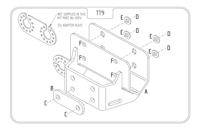
Note: 1. Recommended Torque Setting for M12 Grade 10.9 -139 Nm. (For other Torque Settings see notes overleaf.)
