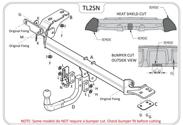
Note: 1. Recommended Torque Setting for M12 Grade 10.9 -139 Nm. (For other Torque Settings see notes overleaf.) 2. Nose load limits and vehicle manufacturers trailer / caravan weight limits must be observed.
