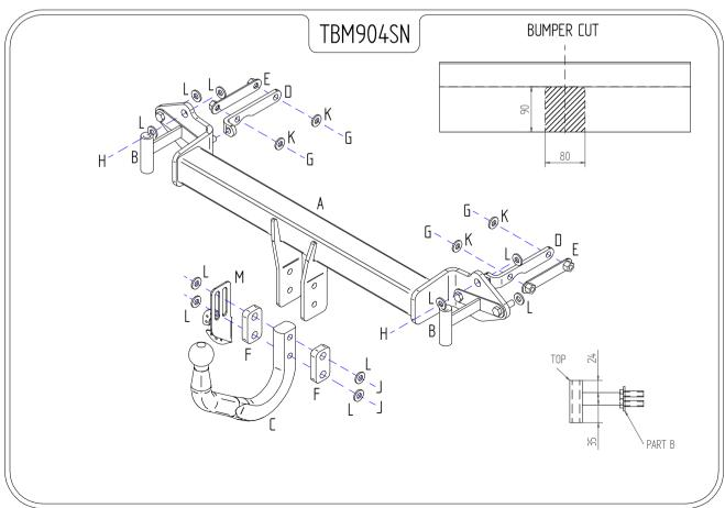
Note: 1. Recommended Torque Setting for M12 Grade 10.9 -139 Nm. (For other Torque Settings see notes overleaf.)
