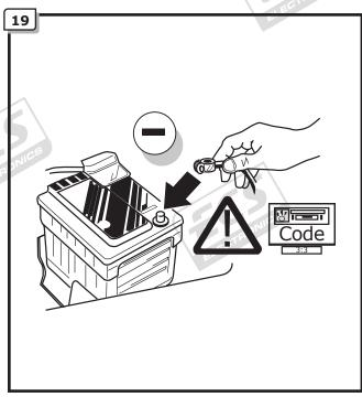
TEST ALL THE CIRCUITS WITH A TEST DEVICE WITH THE CORRECT POWER
