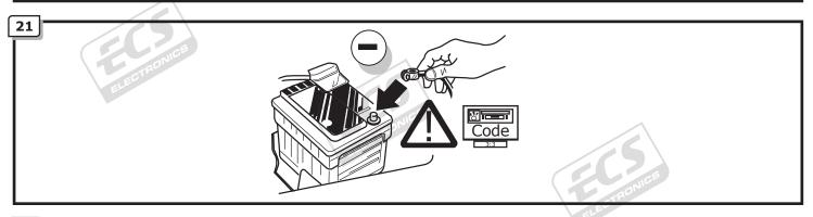
TEST ALL THE CIRCUITS WITH A TEST DEVICE WITH THE CORRECT POWER LOAD FOR EACH FUNCTION. A TEST DEVICE WITH LED'S CANNOT BE USED FOR THIS PURPOSE.
