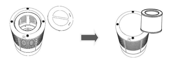
3. After replacing the filter, lock the filter cover by turning it clockwise.
