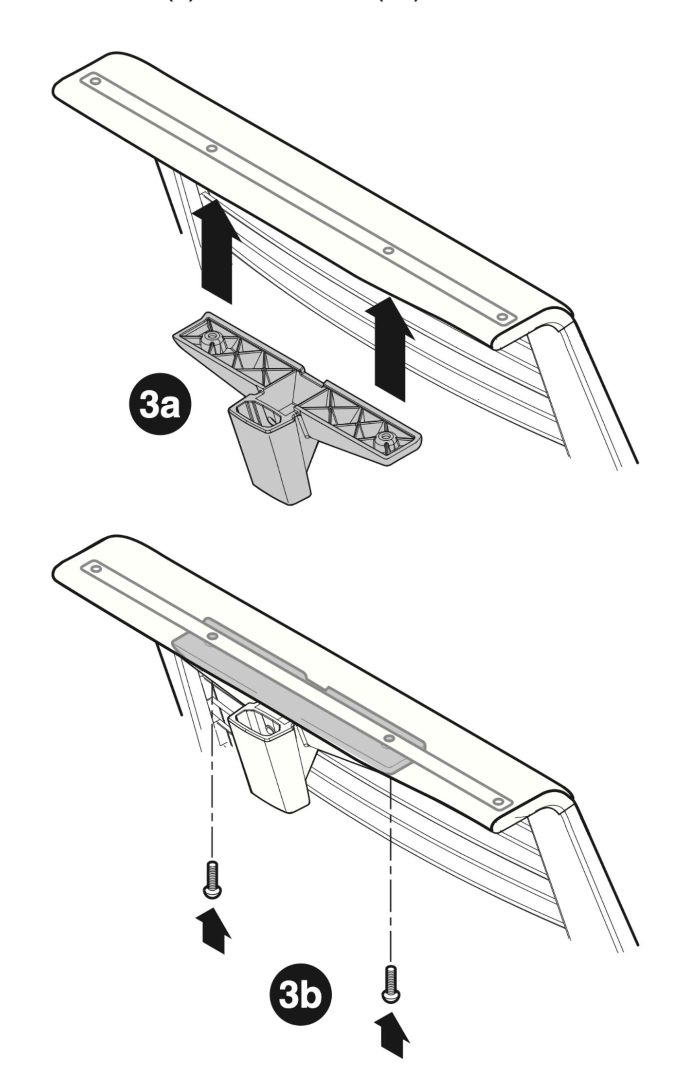
4. Lift the shipping plug out of the headrest support. 5. Slide the headrest arm assembly into the headrest support.
