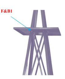
3. Screw the center of B1 to A2 on 4 sides, following the pattern below, install the rest parts; <u>remember to screw B2</u> with a B1 together on A3
