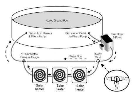
**ATTENTION**: Make sure to completely open the valve (3 holes) in operation.
