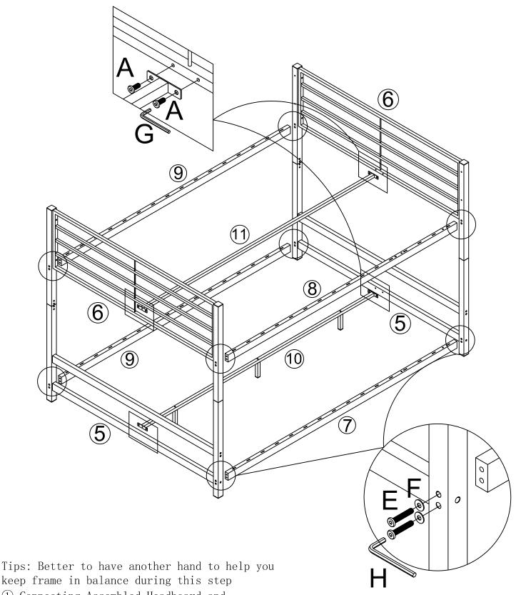
① Connecting Assembled Headboard and Footboard with side bar #7, #8 and #9 by using the Screw E & Washer F (Do not fully tighten now)
