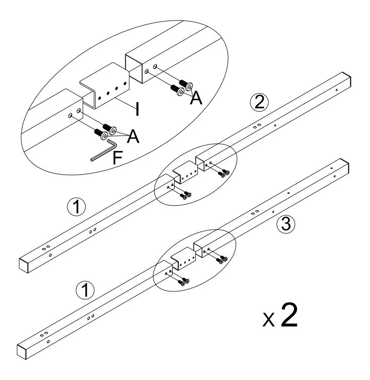
Put U shaped connecting plate I insert Column #1, And then connecting Column #1 with #2 and #3 separately by using Screw A
