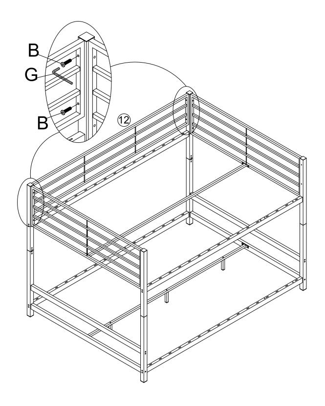
Put Back fence #12 on by using Screw B
