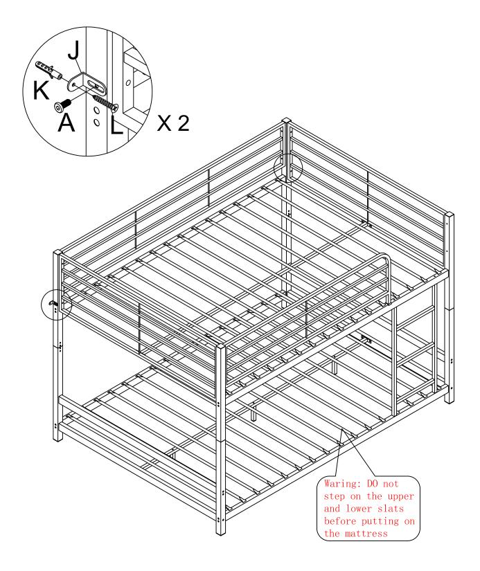
Attach bed to the wall for extra stability by using Connector (J) with Expansion bolt (K) and screw (L) . This step is optional.
