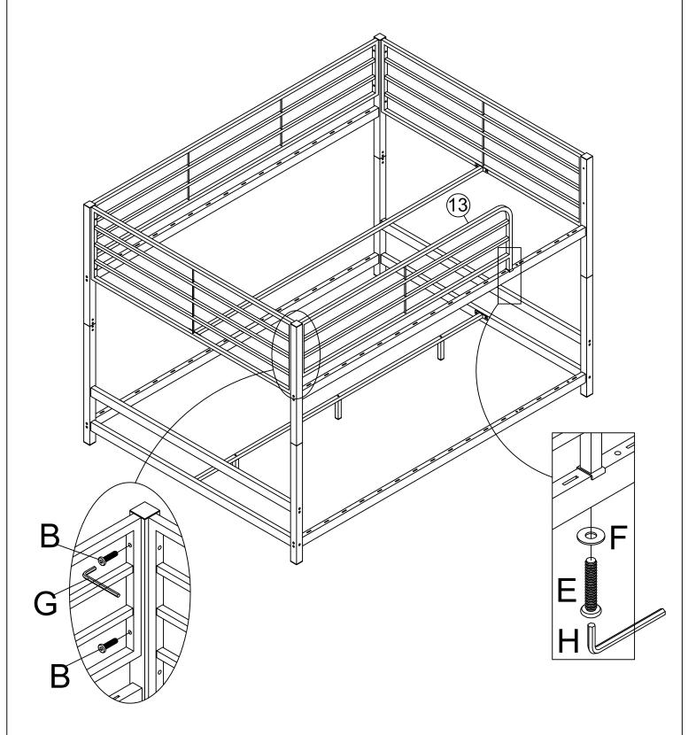
Put Front fence #13 on by using Screw B, Screw E & Washer F
