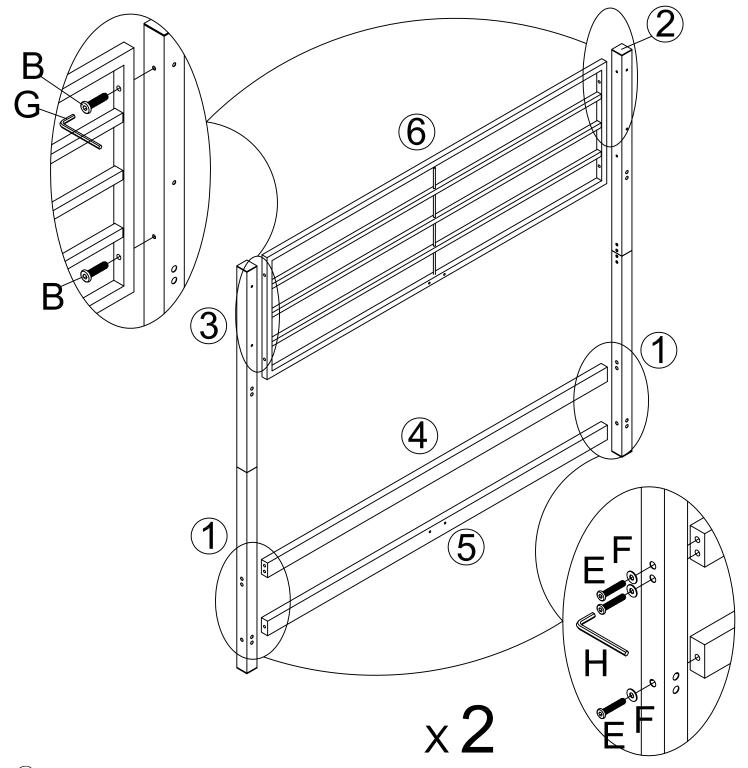
① Headboard: Connecting the Side fence #6 with assembled column via Screw B; and then put on #4 and #5 by using Screw E and washer F
