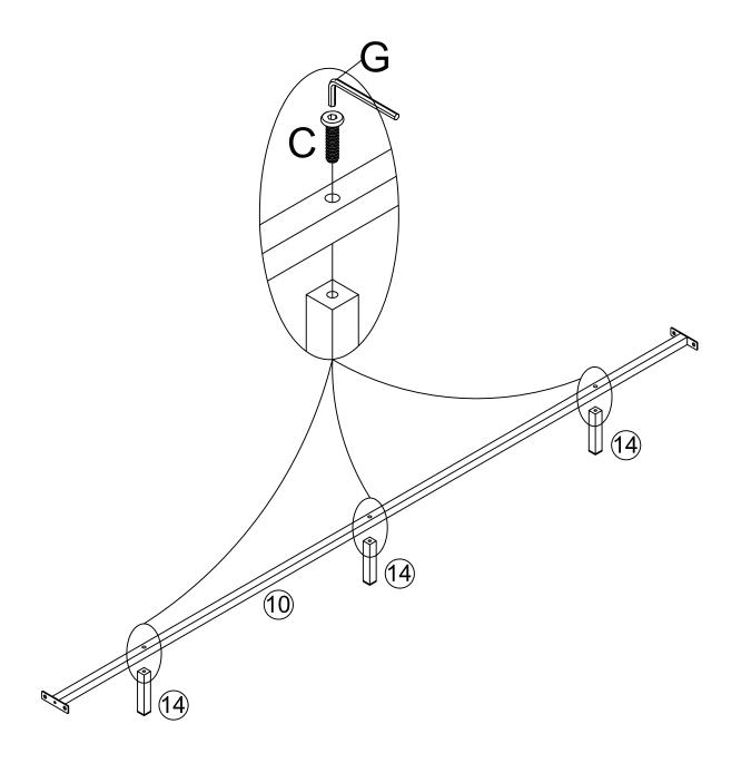
Put Suppot leg #14 on the Bottom center beam #10 by using Screw C
