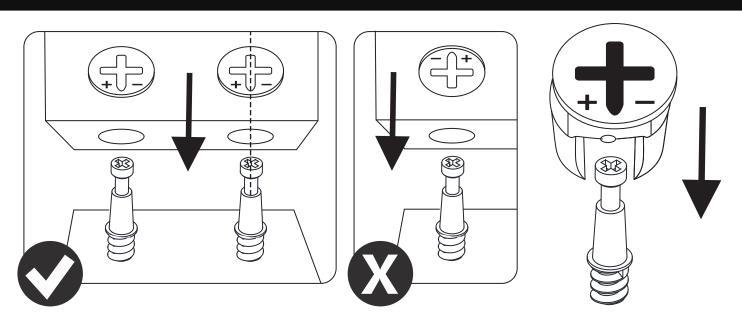
Please place the cam lock according to the direction of the arrow
