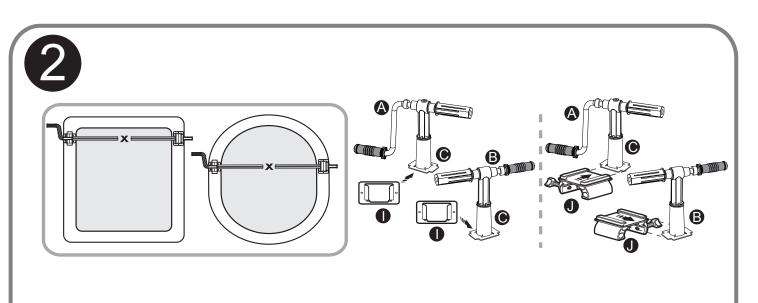
The required length of the tube set is the length "X" from the end of hexagonal tube connector on hub"A+C" to the end of hexagonal tube connector on hub "B+C", when both frames are positioned on each side of pool.
