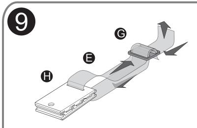
Stick 8 "F" onto the tube at even intervals. Stick belt "E" onto "F". Assemble "H" onto belt "E".
