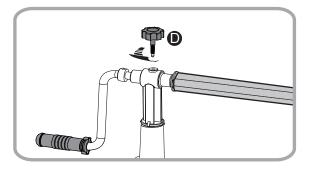
Make sure the screw "D" is screwed into frame "A".
