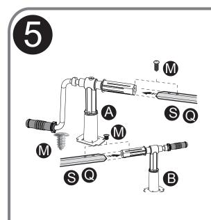
NOTE: The holes on tubes "Q" or "S" should be positioned at both ends of the complete tube configuration, ready for c onnecting the hexagonal tube connectors on "A" and "B".
