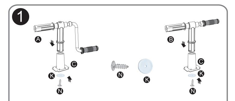
Insert crank frame "A" into frame support "C", secure it with self-tapping srew"N" and plate"K". Insert End frame "B" into frame support "C", secure it with self-tapping srew"N" and plate"K".
