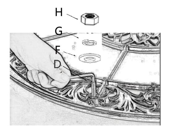
Screw D in and insert the leg. Then put F,G,H on.Please note that don't tighten the screw until you finish the assembly.
