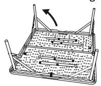
4. Make the connection part in straight and insert the steel pipe
