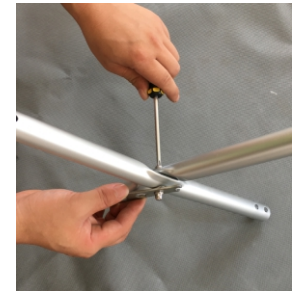
NO.4 Assemble the leg cross-brace Take the two leg cross-braces and place one on top of the other with the grooves properly aligned. Place 2 washers, one on both sides of the cross-braces. Insert screw through washer and into the center hole and secure with a nut.
