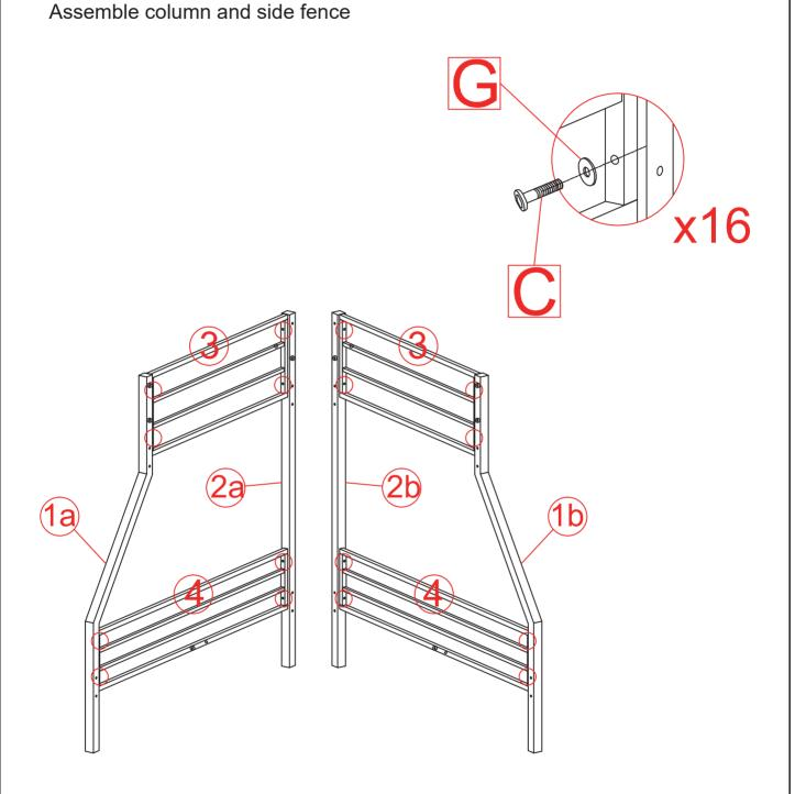
Assembly method: M6x35 screw (C) is screwed from the screw hole on fence inside. Connect fence (3 & 4) to column (1a & 1b & 2a &2b). And pad flat washer (G) between screw and fence.
