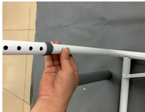
No.2: Insert the leg tube into the supporting bracket in turn and push it to the marble pop.
