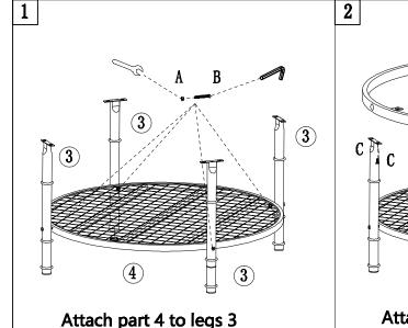
with screws B and nuts A.
