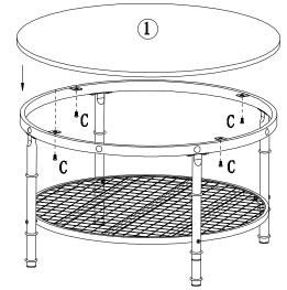
Attach tabletop to frame(from step2) with screws C.Adjust and tightenall screws and make sure table does not wobble.
