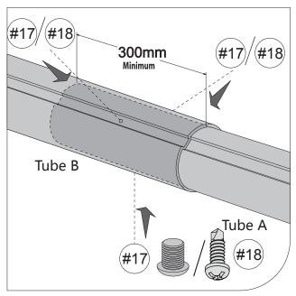
• If you have a screw driller, you could use #18 screws, if not, please use #17 screws. We suggest you use #18 screws to fix it in case #17 screws fall out the tube when use it for a long time.
