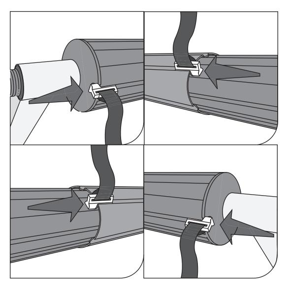
• Please note slight movement of the strap is normal because the flexible straps are design to ensure the force to be even when roll up or out the cover.
