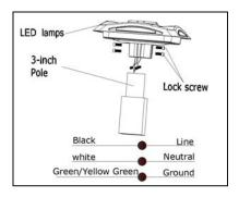
1) Connect the AC wire of the lamp as shown in the picture, then insert the lamp into the 3-Inch pole.
