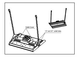
2) .when the chain length adjusted ok, Put fixture fixed on Hooks. Fasten the lock rope.
