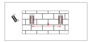
1. Mark the bracket install hole's position on the wall. The distance is 280+/-20 mm for 2FT and 830+/-20mm for 4FT.
