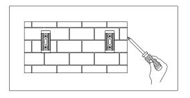
2.Drill the holes and screw on the bracket of the wall
