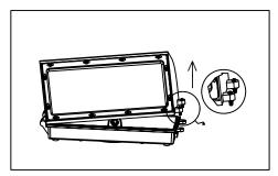
3). Connect wire A with wire C (The black one is L, white one is N, and the yellow one is ground wire), installing the front cap.
