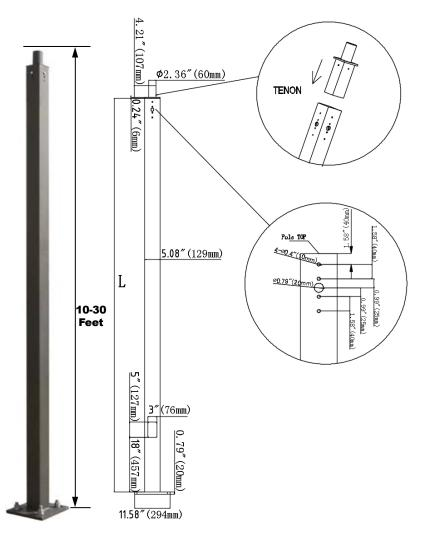
The WISDOM Series Straight Square Steel poles are built from high strength steel tube and are available side drilled for arm mounted area lighting luminaires or with tenon mounts for flood and post top luminaires. Typical area lighting applications include retail centers, industrial parks, schools and universities, public transit and airports, office buildings and medical facilities. Mounting heights of 10 to 30 feet can be used based on selected luminaire application.
