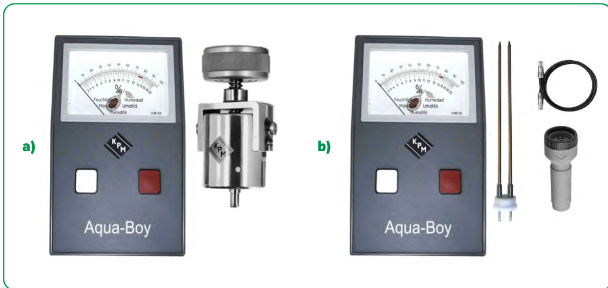
Figure 49. a) Cacao-specific moisture metre Aqua-Boy KAM III with cup electrode 202 and b) stab electrode 209 b, cable and holder. ( aqua-boy.co.uk ).
