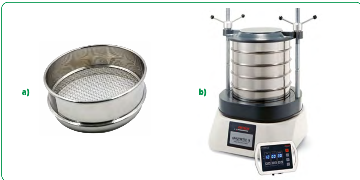
Figure 53. a) Test sieve for separating cacao beans from dirt particles; b) mechanical sieve shaker for bean size distribution measurement and analysis ( lavallab.com ).
