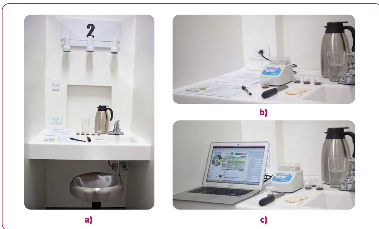
Figure 17. a) Sensory evaluation booth equipped with samples, printed evaluation form, spatula and water thermos b) with heating equipment; and c) with heating equipment and computer with evaluation form (Bioversity International, Archila, 2022).
