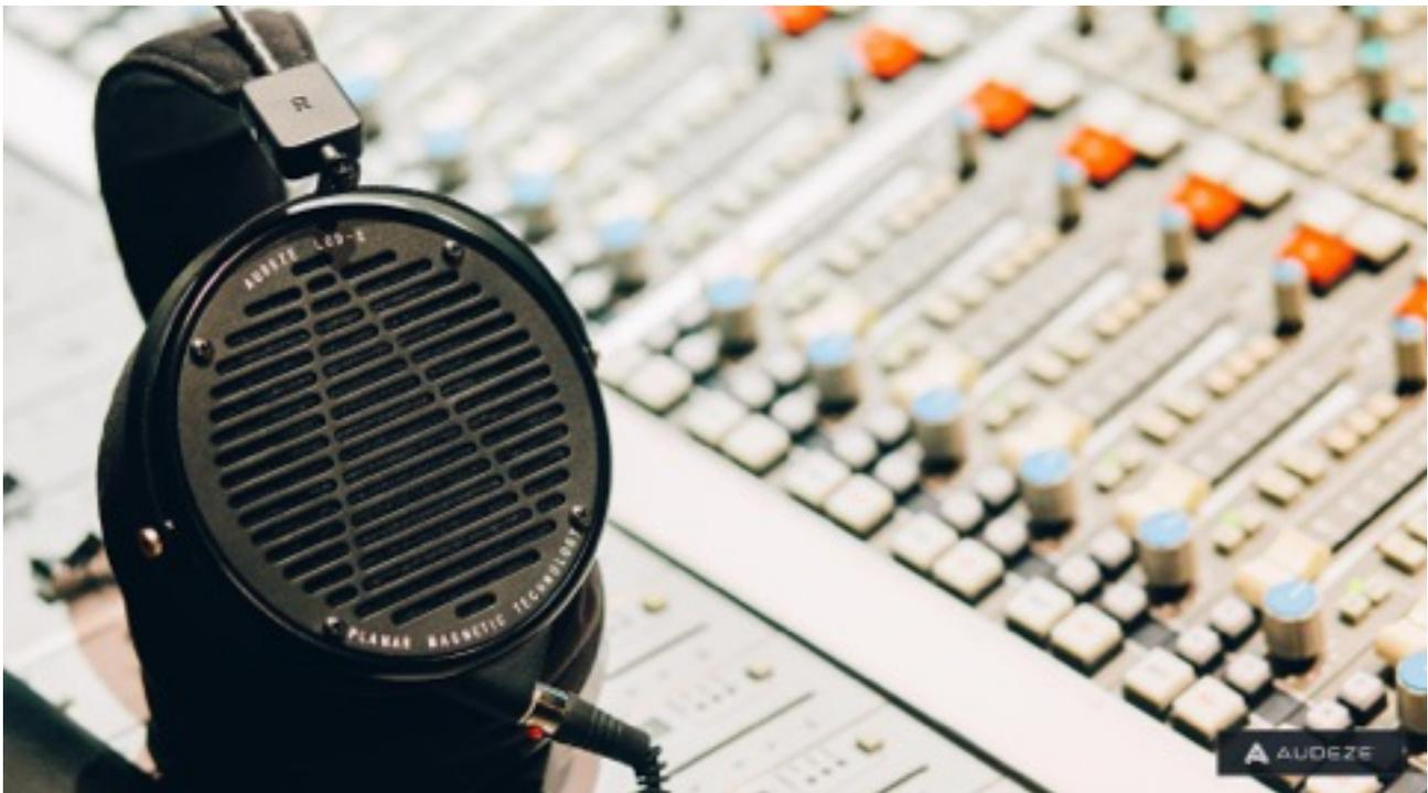
The Audeze LCD-X headphones come in a rugged plastic equipment case, with a nice complement of cables and adapters. The model's open-back earcups house planar magnetic drivers with ultra-thin diaphragms (thinner than a human hair). Claimed frequency response is "5 Hz – 20 kHz, extended out to 50 kHz." The ear pads are premium, butter-soft leather; and they even make what they humorously and unofficially call the "vegan" version, which utilizes microfiber suede instead of leather.
