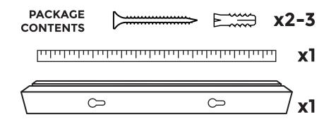
TO INSTALL, Tape ruler to the wall, making sure to be level. Place shelf against ruler where you would like it mounted, marking the center of small end of slot (16" apart). Drill through the wall at each point and insert the anchors before installing each screw about 1/4" out from the surface.
