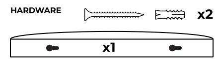
**TO INSTALL,** Cut along dotted line below and tape guide where you want your Micro Ledge, making sure to be level. Drill through crosshairs, insert anchors and install screws – **fine-tune screw depth for a snug fit.**
