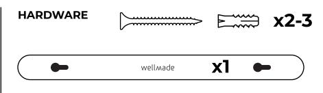
**TO INSTALL,** Mounting holes are 14" apart. Making sure to be level, mark the center of where you want your Photo Rail and measure outward. Drill a 3/16" hole, insert wall anchors and install screws about a 1/4" above the surface. **Please note, fine-tuning screw depth is crucial to functionality.**
