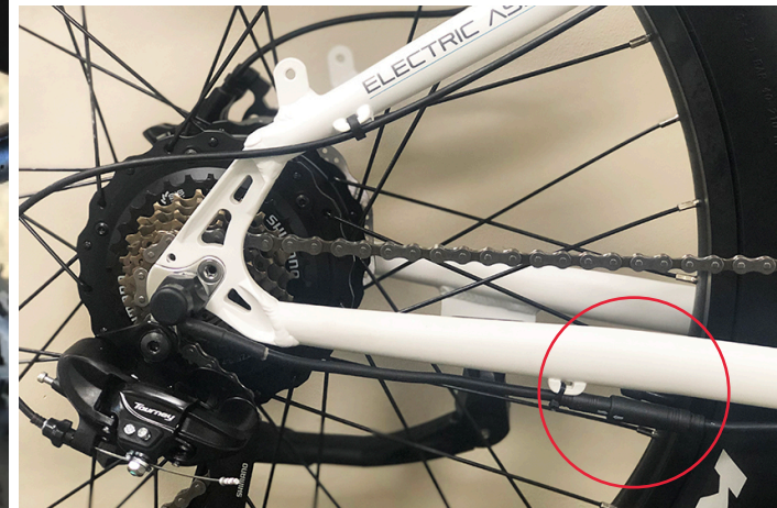
Fig. 2 Quick Disconnect (Rear frame section)
