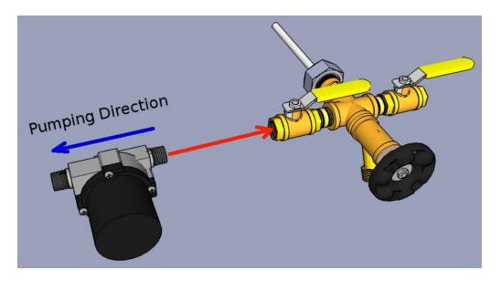
The pump should end up oriented as shown in the picture. The pumping direction is very important for the efficiency of the system. There is always a marking on pumps which indicates in which direction the pump moves the water. This must be AWAY from the bottom feed connector. You should NOT use the included blue sealant on the pump. Instead use the included Teflon tape. Use at least 7 wraps of the tape on both sides of the pump.
