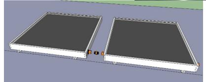
Start threading the union into the nuts on one panel and hand tighten only to allow some flexibility when lining up the panels. Bring the panels close to each other so the nuts on the second panel can be threaded onto the union, hand tighten. Slightly tighten the nuts on both sides. Not much torque is needed to form a tight seal. Once the system is pressurized you can tighten until all leaking stops.
