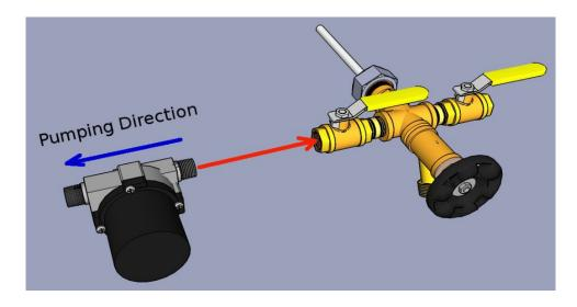
The pump should end up oriented as shown in the picture. The pumping direction is very important for the efficiency of the system. There is always a marking on pumps which indicates in which direction the pump moves the water. This must be AWAY from the bottom feed connector. You should NOT use the included blue sealant on the pump. Instead use the included Teflon tape. Use at least 7 wraps of the tape on both sides of the pump.
