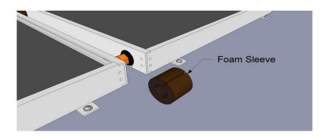
Install a foam sleeve over every fitting between panels as well as at the ends of the panel array.
