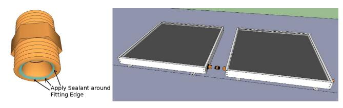
Start threading the union into the nuts on one panel and hand tighten only to allow some flexibility when lining up the panels. Bring the panels close to each other so the nuts on the second panel can be threaded onto the union, hand tighten. Slightly tighten the nuts on both sides. Not much torque is needed to form a tight seal. Once the system is pressurized you can tighten until all leaking stops.
