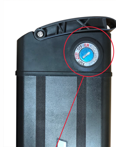
Battery lock switch
