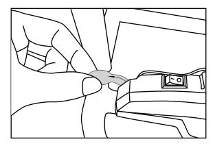
Pull out the insulating strip to start using the tail light
