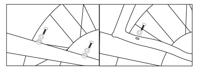
Remove the 4 allen bolts and washers from rear fork. Put on rack. Fasten the bolts securely.
