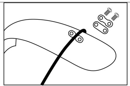
4, Mount front fender to front fork with 2x allen bolts on each side
