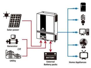
Figure 1 Basic hybrid PV System Overview
