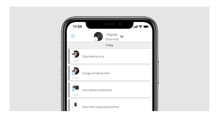
When a Tag or Pass is linked to a user, it fully inherits the rights to manage the user's security modes. For example, if a user was able to manage only one group, then the bound Tag or Pass will have the right to manage only this group.
